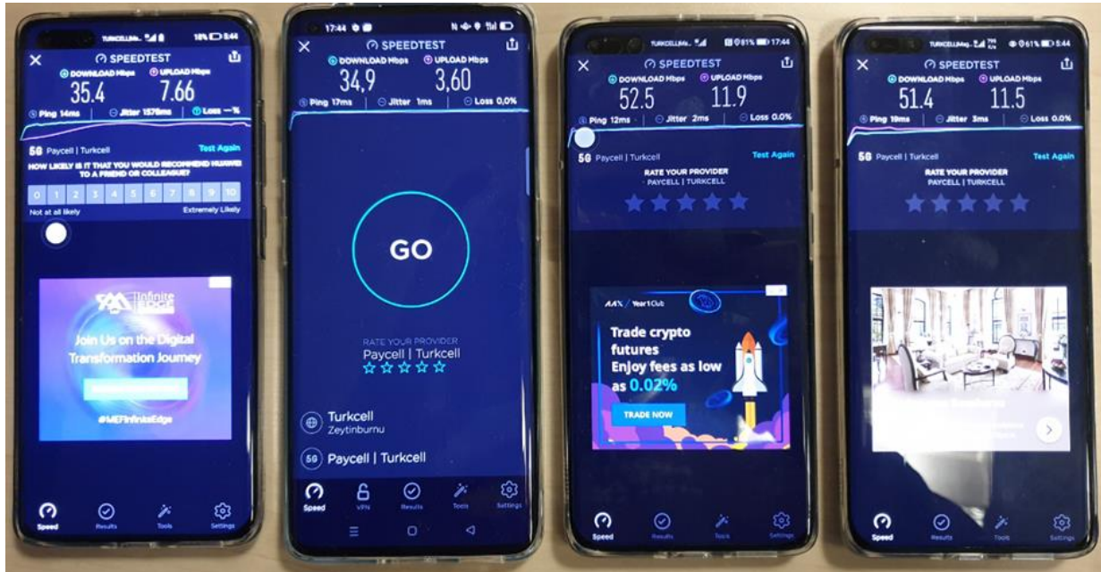
Figure 4: Slice #1 Terminals (UE1 and UE2) on the Left Side Approximately Get 1,5 times Lower DL Throughput than Slice#2 Terminals (UE3 and UE4) on the Right Side after Resource Reservation to Slices.
