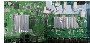
10G Transmission board
