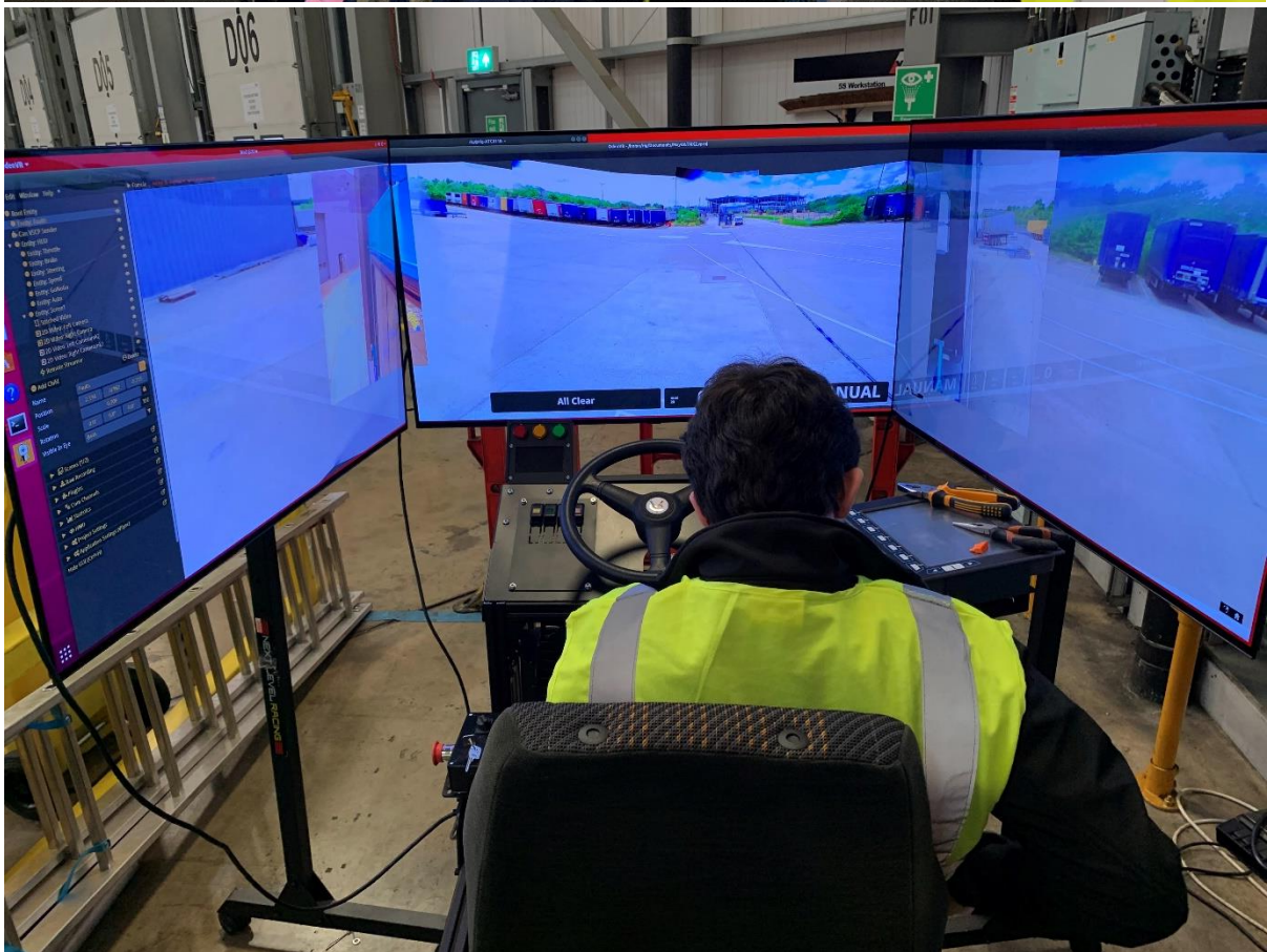
Fig. 13. Remote drivers in the teleoperation unit
