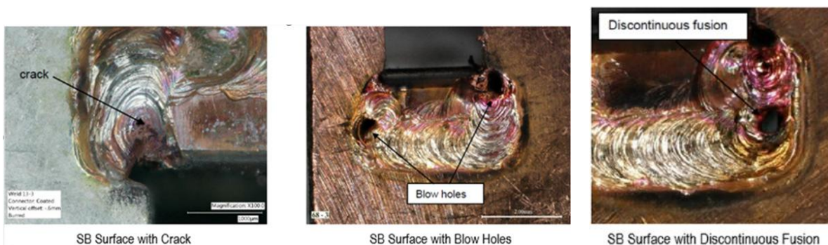
Figure 18: images showing weld defects
