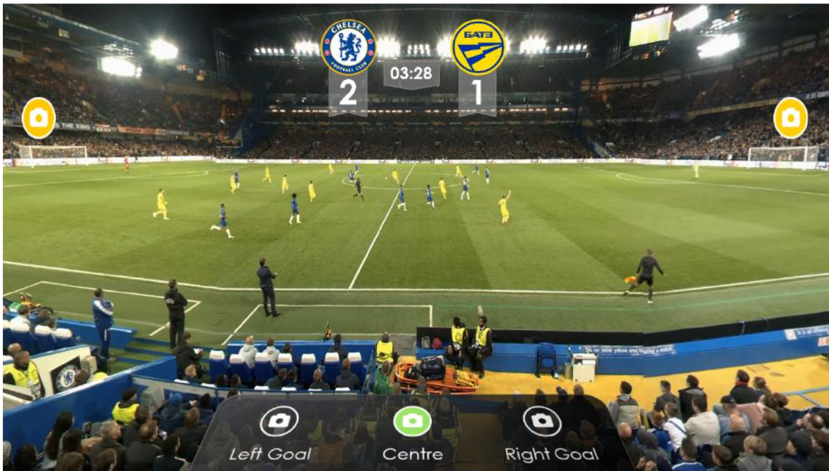
Figure 6 Guide image for the 8K 360 football use case. The illustration shows the viewpoint, that may be shown in a VR headset or a flat screen device (tablet), from an 8k 360 camera positioned at the half-way line of a football match, showing interaction options at the bottom of the screen that give the user option to 'jump' to an alternative camera position.
