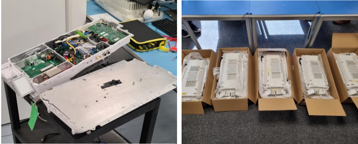
Figure 7 - CoMP-O-RAN Small Cells in manufacture and assembly
