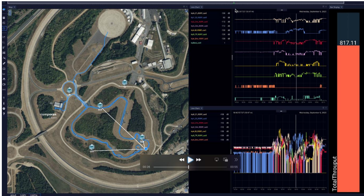
Figure 24 - Cloud-based telemetry tracking UE location with TRP measurements.
