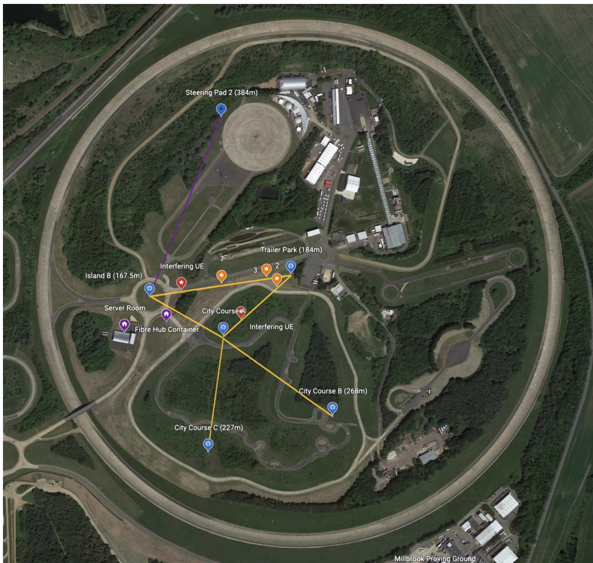
Figure 19 - Pole locations used for the CoMP-O-RAN Cell
