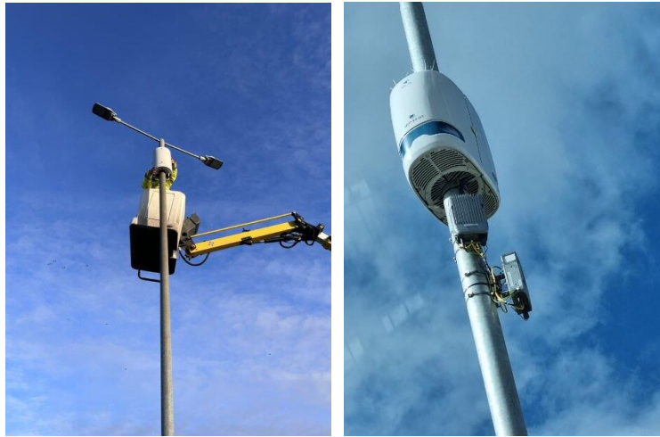
Figure 17 - Early CoMP-O-RAN small cell prototype at TV5G with external mmW
