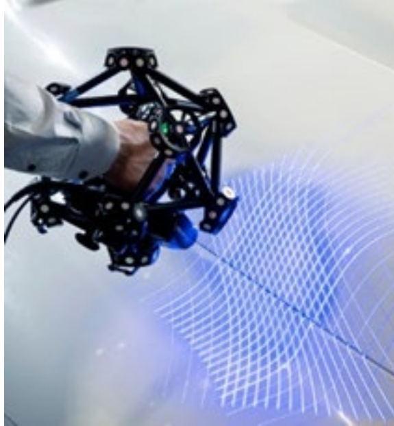
Figure 21 - Mobile Robot use case: Metrascan scanning the aircraft for digital twin
