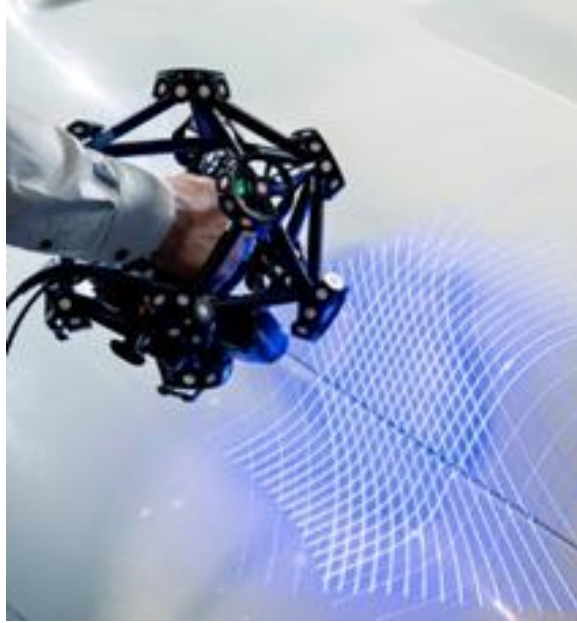
Figure 22 - Mobile Robot use case: Metrascan scanning the aircraft for digital twin
